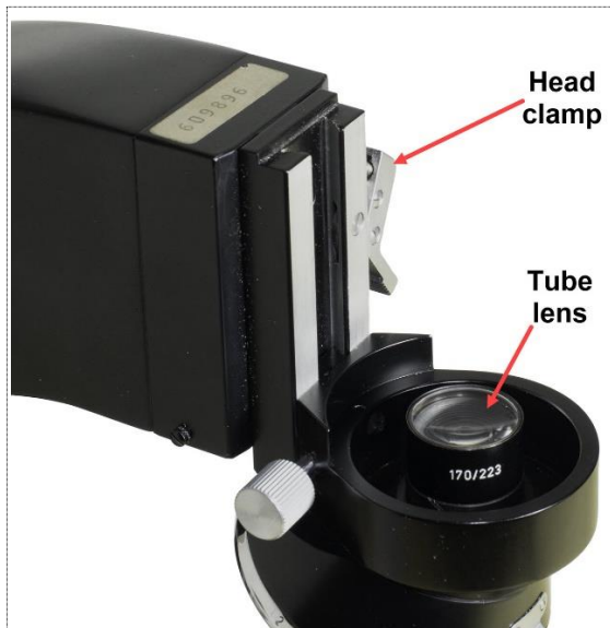
Figure 26: Ortholux nosepiece with its tube lens.
