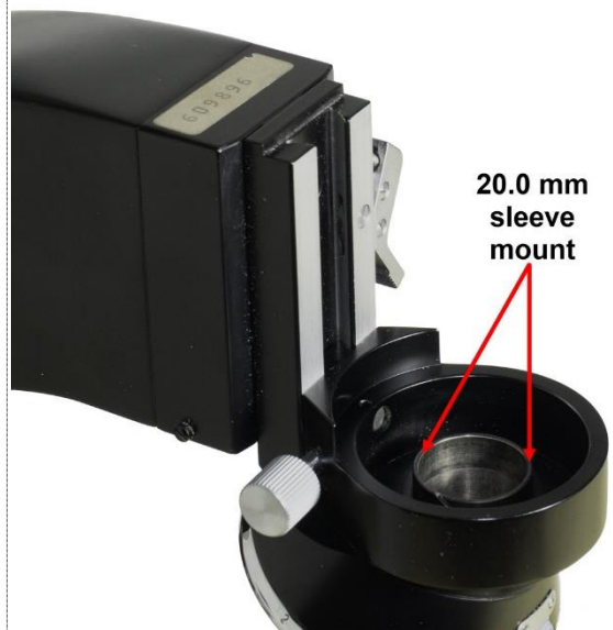
Figure 27: Ortholux nosepiece with removed tube lens.
