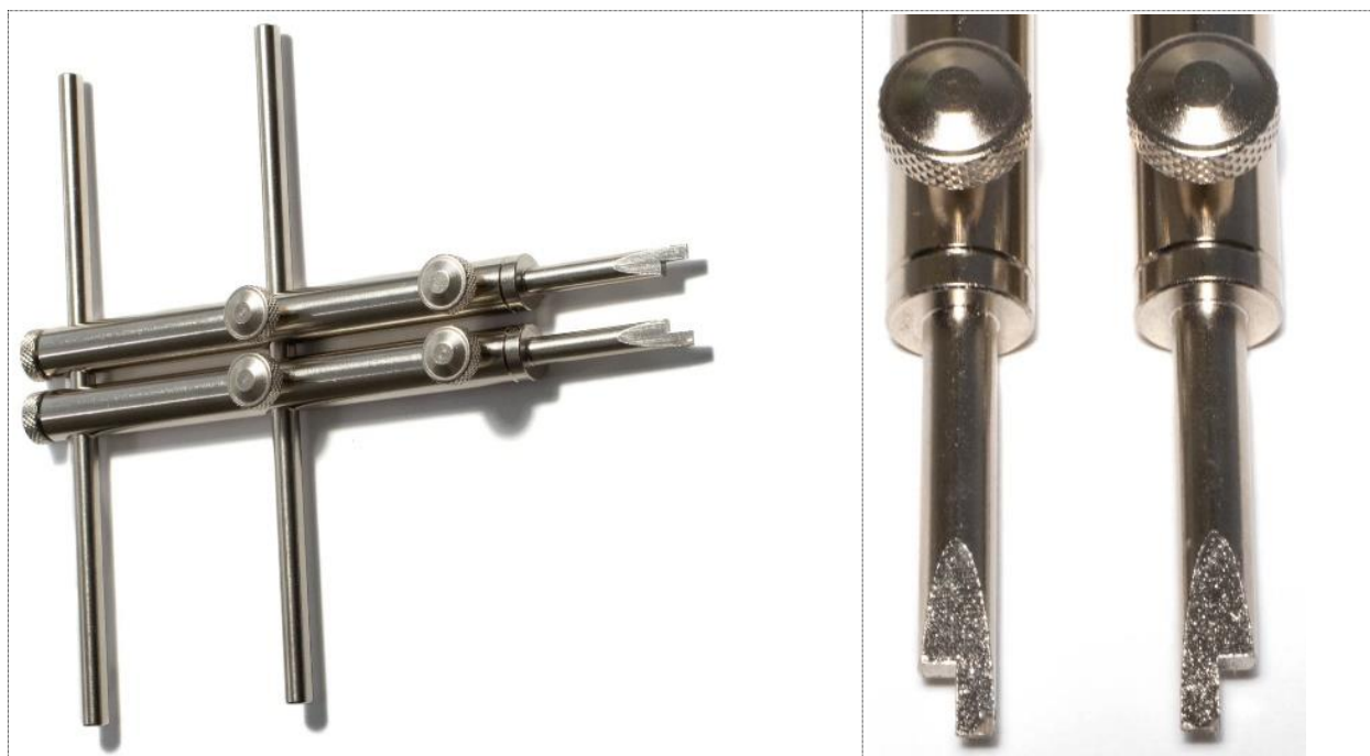
Figure 8: An example of a suitable camera lens spanner. To the right is a closeup of the required flat screwdriver type tips.
