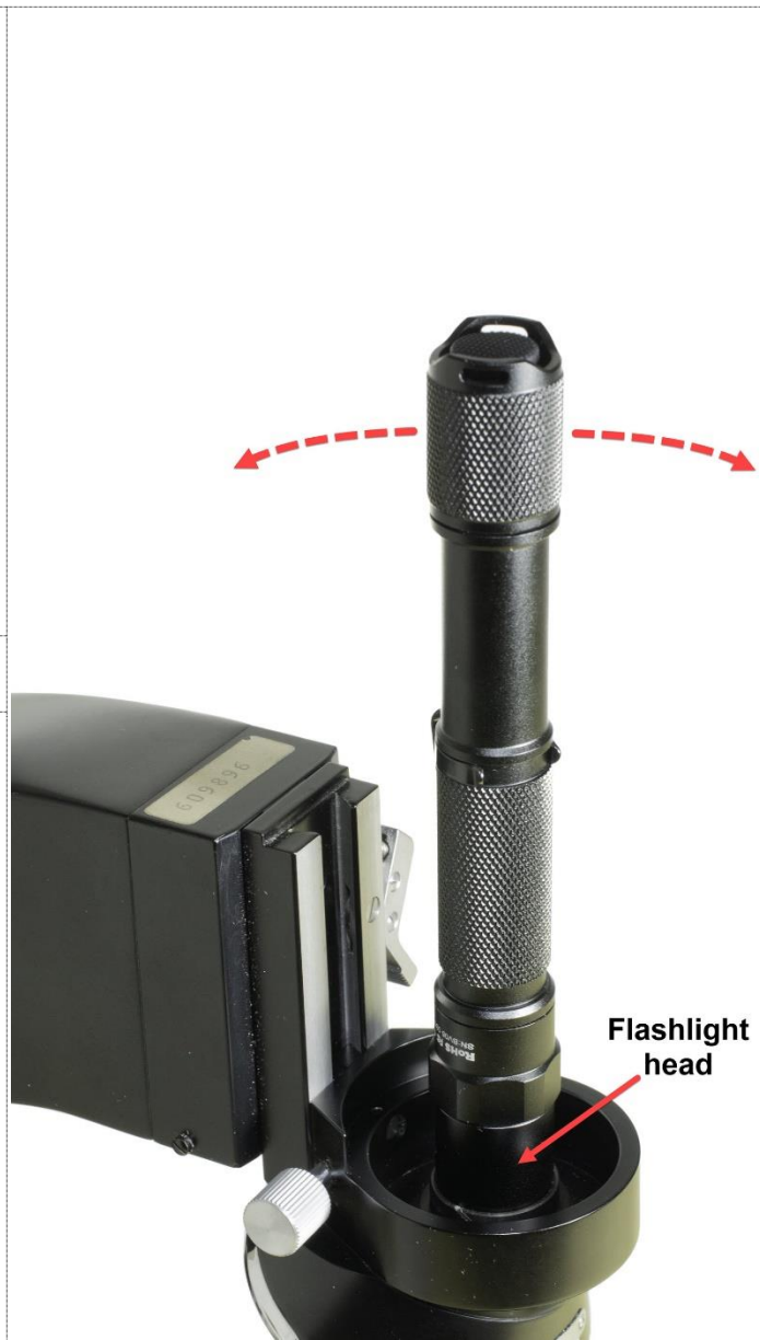
Figure 28: Ortholux nosepiece with attached flashlight.
