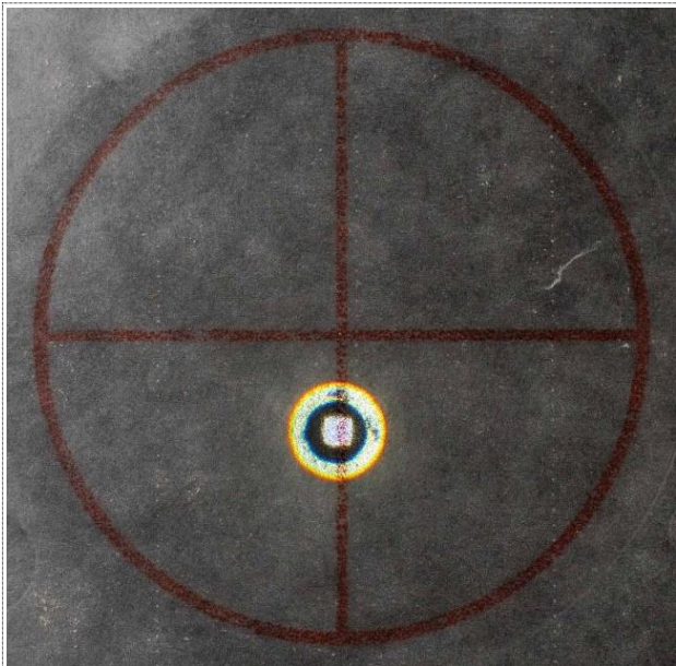
Figure 31: The light dot is clearly off the target which indicates that the mirror plate and/or the mirror & swing-out lens holder require adjustment.
