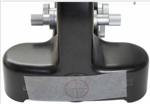
Figure 25: The lamphouse port symmetrically covered with the collimation target wax paper printout.
